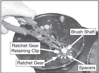
Figure 13. Ratchet gear assembly.
